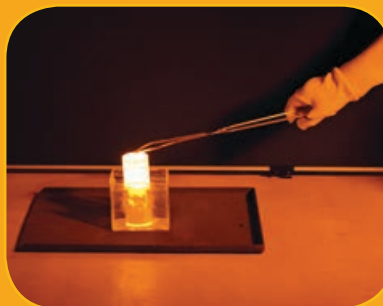
Thermal shock test of a 1200 °C hot burner nozzle in water.
