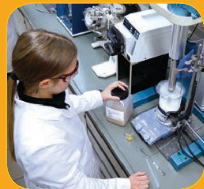
Preparing the ceramic slurry in the laboratory of the University of Bayreuth.
